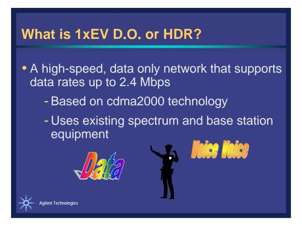
1xEV D.O. is a high-speed, data only network that supports data rates up to 2.4 Mcps and is based on cdma2000 technology. This system operates in existing spectrum, utilizes existing base station equipment with upgrades, and is on the fast track to reach the market. The 3GPP2 standards body spent only 6 months developing Release 0 of 1xEV D.O.
