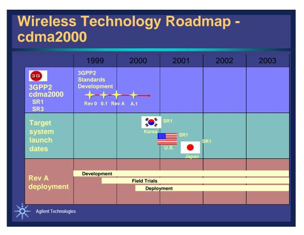
Within Korea and the US cdma2000 is going to undergo a rapid rollout. The cdma2000 technology can be considered to be an upgrade to the existing IS-95 systems. IS-95 network operators will be able to convert existing systems from IS-95 to cdma2000 by installation of new cards in their current base stations without the need for investing in totally new equipment. The conversion of handsets from IS-95 to cdma2000/IS-95 will be very quick once service starts.
