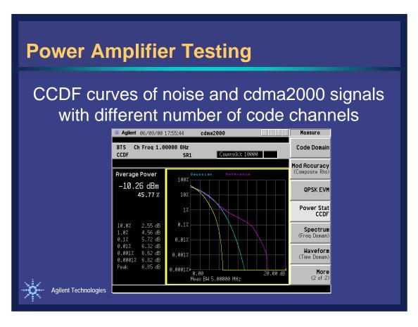
This is a measurement of 2 different cdma2000 base station signals. The blue line in the center is Additive White Gaussian Noise for comparison. The plot on the left is the base station signal containing only a few code channels. The plot on the right is a fully loaded base station signal.
