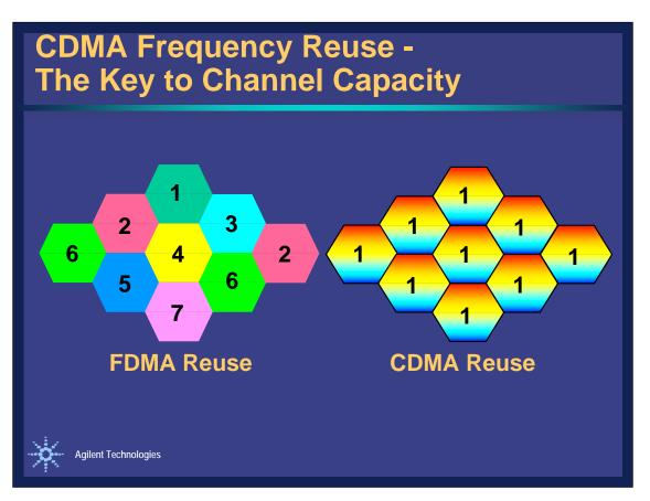
The major capacity advantage of CDMA is realized by many technical innovations. One of the most important is the reuse of the same frequency in every sector of every cell. In IS-136 and analog cellular systems, there is a 7 cell repeat factor, with 3 sectors. This means that only one out of every 21 channels is available to each sector. GSM usually uses a repeat of 4, with 3 sectors, for a reuse of one out of twelve.
