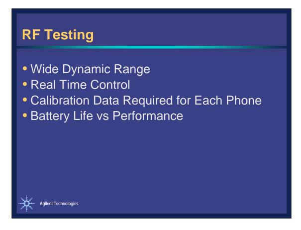
There are several differences in CDMA technologies from analog or either of the TDMA technologies. One of the biggest difference is the dynamic range requirement. GSM phones operate over no more than 40 dB transmit power range. CDMA phones have to operate over a much wider range, up to about 80 dB. In addition, there are design specs on the accuracy of this level, as well as the accuracy of the phone to measure the receive level over this entire range.
