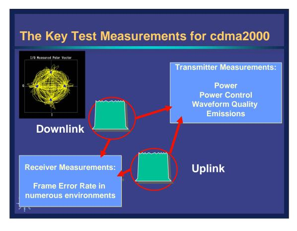
The important RF measurements for CDMA are shown here
