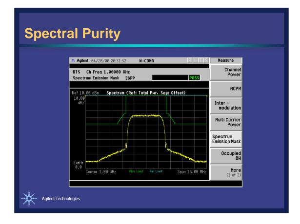
It is too expensive to have a power amplifier (PA) with 16 dB overhead. For a base station with 25 watts average power, this is 1 kilowatt of peak power. Instead, if we allow the base station to clip 0.1% of the time, the peak power can be reduced to only 260 watts. Whether this is acceptable depends on the spectral density outside the desired channel.
