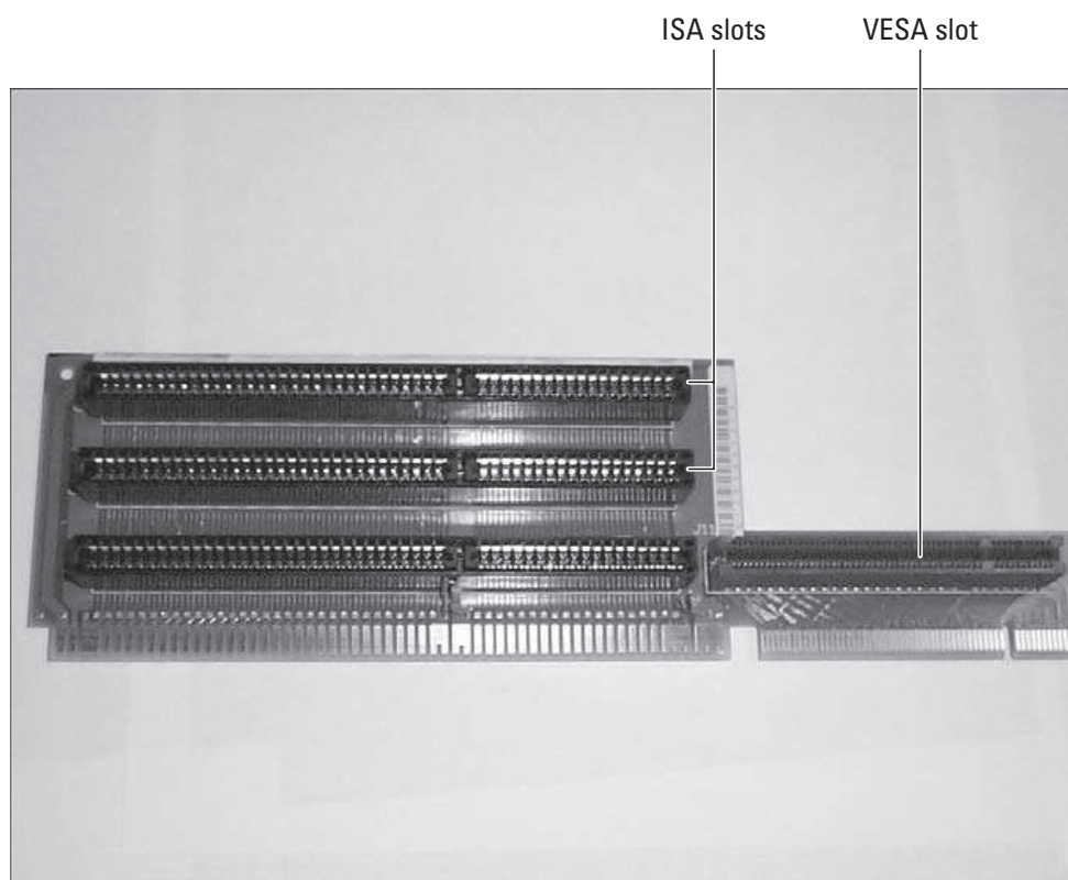
Figure 1-40: Looking at a VESA slot, which is an extension of the ISA slot.
