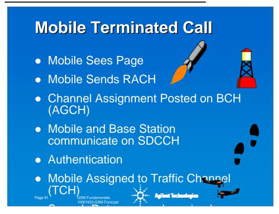
The process for base station originated calls is very similar. The base-station posts a PCH (paging CHannel) on the CCCH part of the BCH. When the mobile receives the PCH, it responds by sending a RACH. The remainder of the process is identical to the mobile originated case.
