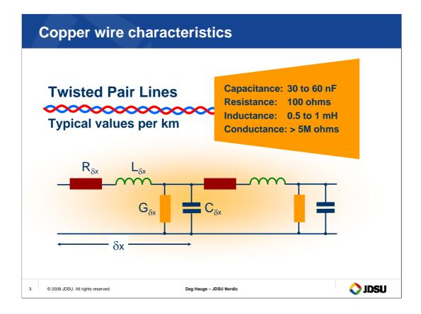
Paired telephone cables, for example, are made up of a few to several thousand twisted pairs. However, the copper strands have a slight amount of resistance as well as a small amount of capacitance and inductance, which causes impedance when put together. In other words, it holds back the flow of the electrons and signal.
