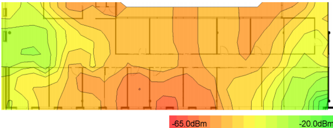
Figure 112 - Partial signal strength measurement example.
