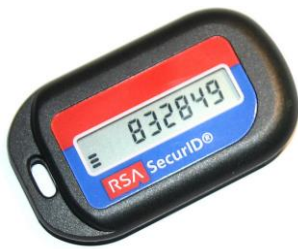
Figure 93 - Security token using time synchronized one-time-passwords
