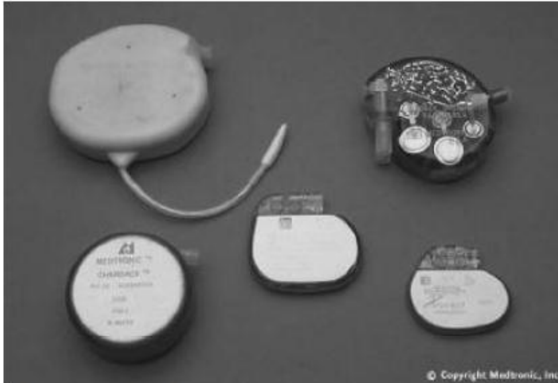
Figure 13.6 Examples of early pacemakers (top row) and metal encapsulated devices (bottom row). The two units on the bottom right are modern pacemakers that are about the size and mass of a pocket watch. (Photograph courtesy of Medtronic Corp.).
