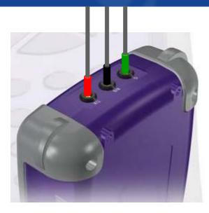
Connect the 3 test leads to the mini-Banana connectors on the top:
