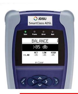
You measure longitudinal balance to: check if the pair's A and B are electrically the same in their ability to cancel noise.
