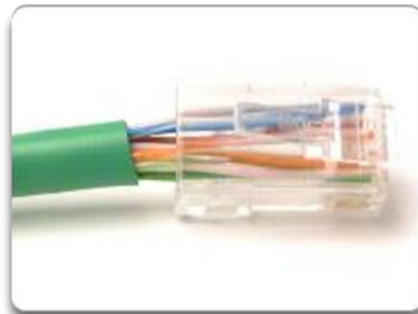
Bad connector - Wires are exposed, untwisted, and not entirely covered by the sheath.
