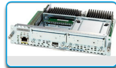
Cisco Wireless Controller on the Cisco Services Ready Engine (SRE)
